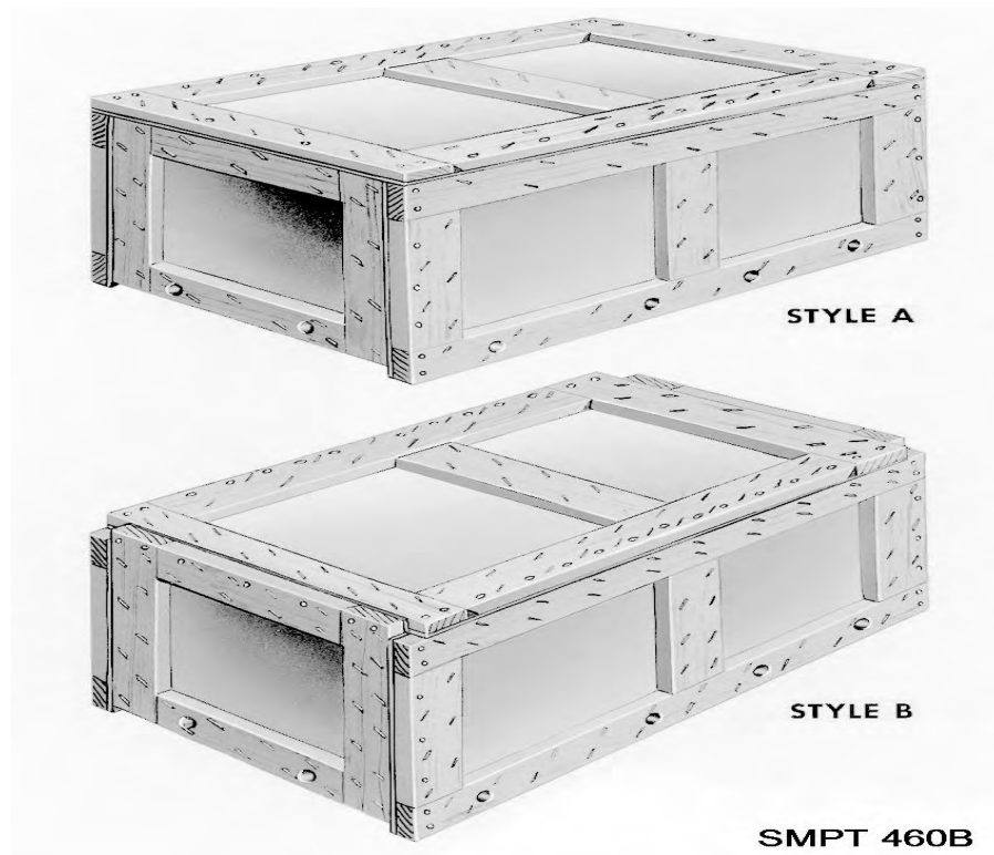
Figure 3-26. Styles A and B cleat arrangement for wood cleated, skidded, loadbearing base boxes.
