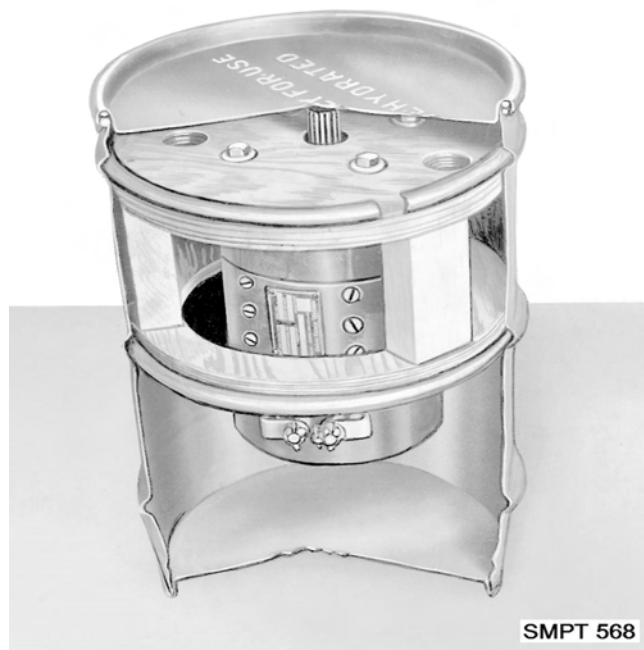
Figure 5-2. Internal locking rings in position (MIL-D-6054).
